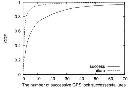
Figure 1: The CDF curves of the lengths of GPS lock *success* and *failure* periods in the Yushan traces
