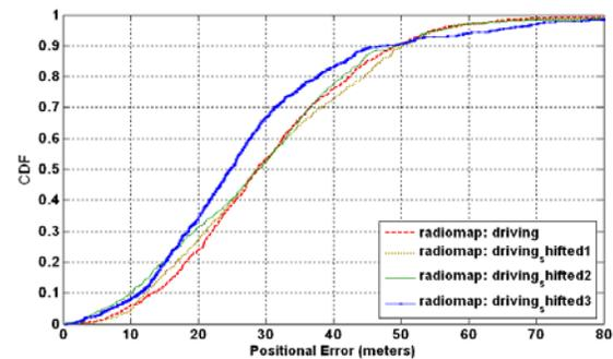
Figure 3. Effect of the GPS delay on accuracy.
