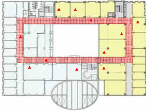
**Fig. 6.** Floor layout for the experiments. The red triangulations are locations of IEEE 802.11 AP and the rectangular area is the corridors of the floor.
