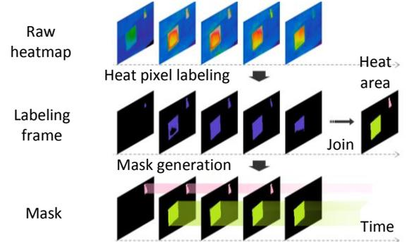
**Figure 6. Appliance mask generation steps. The top row includes raw heatmaps captured in five adjacent times. The middle and lowest rows represent the corresponding labeling frames and masks. The right-most frame contains the resulting appliance heat areas for a lamp and a monitor.**
