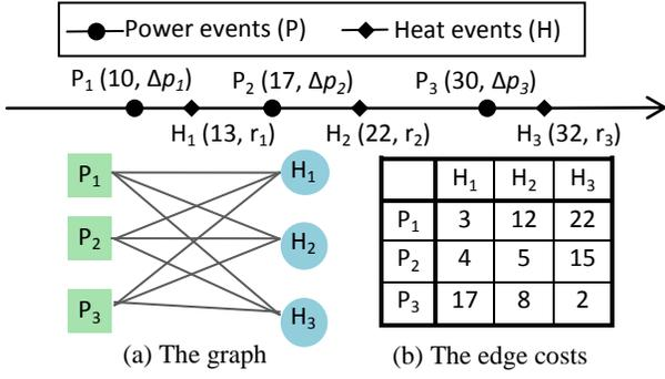
**Figure 9. An example power-heat matching graph. In (a), three power events (P<sub>1</sub>, P<sub>2</sub>, and P<sub>3</sub>) are connected with three heat events (H<sub>1</sub>, H<sub>2</sub>, and H<sub>3</sub>) with edges with costs listed in (b).**
