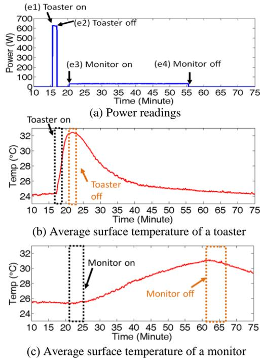
**Figure 2. Resulting average surface temperature of two exemplar appliances (a toaster and a monitor) when the appliance is turned on/off. These two cases show that surface temperature increases (decreases) when the appliance turned on (off).**
