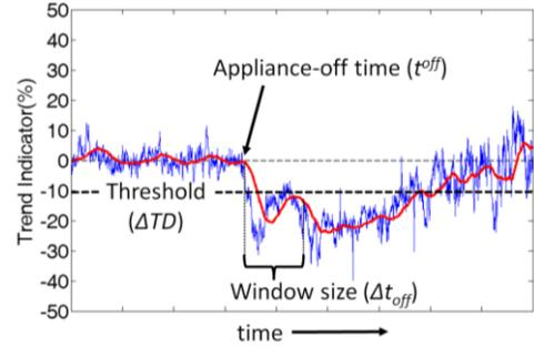
**Figure 8. The trend indicator for an appliance heat area. The blue line is the original data curve, and the red line is the smoothed curve after applying a low-passed filter.**
