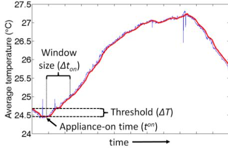
**Figure 7. The average temperature for an appliance heat area. The blue line is the original data curve, and the red line is the smoothed curve after applying a low-passed filter.**
