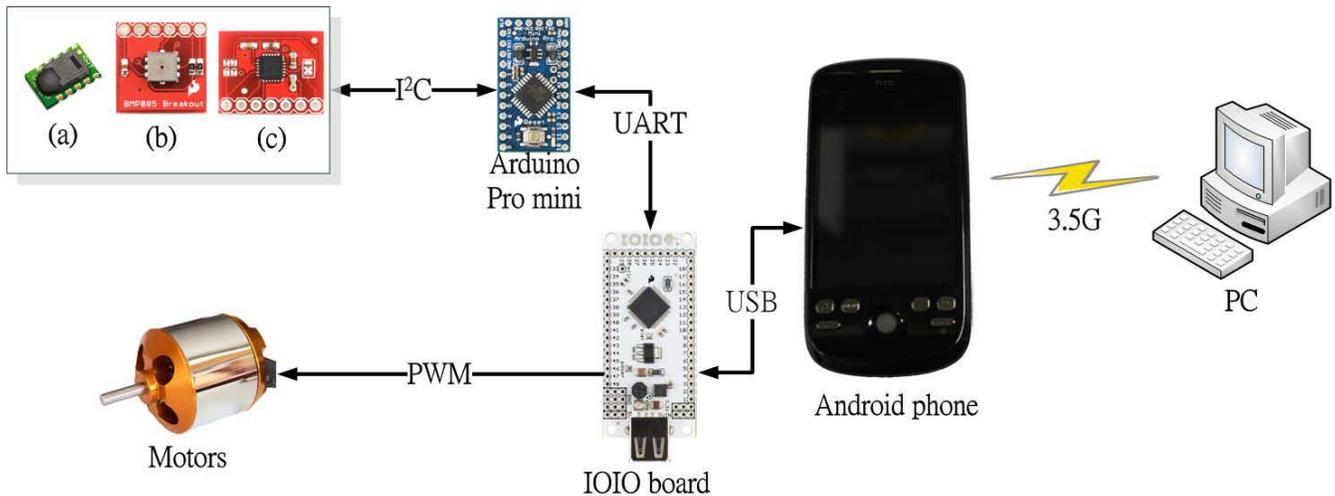
Figure 2. System overview. (a) temperature and humidity sensor - SHT11. (b) barometric pressure sensor - BMP085. (c) three-axis gyroscope - ITG-3200.
