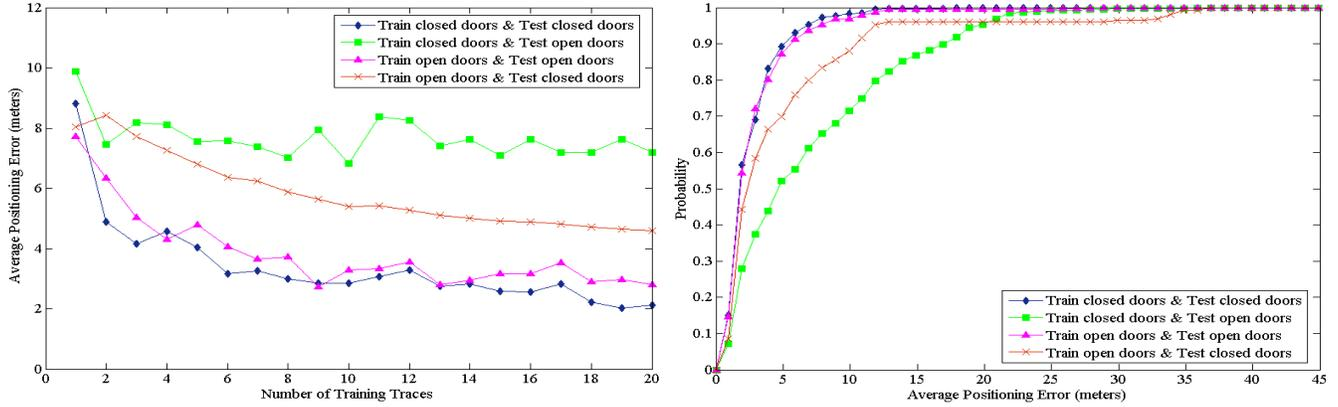
**Figure 8.** The left graph shows the impact of open/closed doors on the average positioning errors under different map-environment combinations. The right graph shows CDFs of their average positioning errors with increasing training samples.
