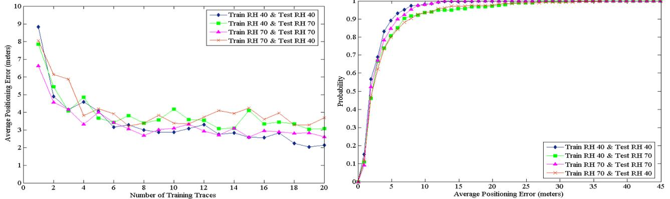
**Figure 10.** The left graph shows the impact of humidity (40% and 70% RH levels) on the average positioning accuracy under different map-environment combinations. The right graph shows the CDFs of their average positioning errors with increasing numbers of training samples.
