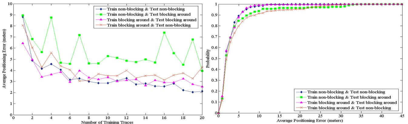
**Figure 9.** The left graph shows the impact of people on the average positioning accuracy under different map-environment combinations. The right graph shows CDFs of their average positioning errors with increasing training samples.
