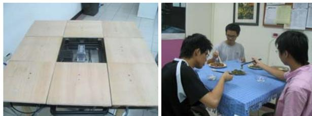
Fig. 5. The picture on the left shows the embedded RFID and weighing table surfaces, and the picture on the right shows a dining scenario.
