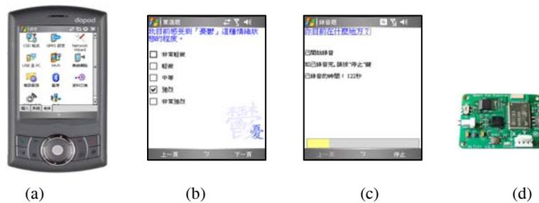
Fig. 7. CoESM tool: (a) Dopod p800w PDA phone, (b) prompted questionnaire of CoESM in Chinese, translating into English is “please indicate to what extent you feel right now”, (c) voice recording screenshot, (d) Bluetooth wireless accelerometer from SparkFun.
