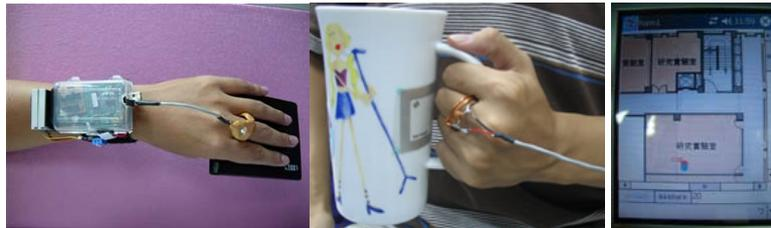
Fig. 4. The object reminder system. On the left shows the wearable wristband device. In the middle shows the RFID tag on the object. On the right is a map display showing the locations of objects.
