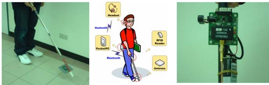
Fig. 3. In iCane, the standard white cane is equipped with a PDA, an antenna, Bluetooth headset and an RFID reader.
