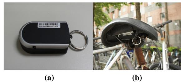
Figure 2 (a) the Bluetooth device (b) mounted to a bicycle. We used a keychain and double-sided tape to lock the tag underneath the Bike
