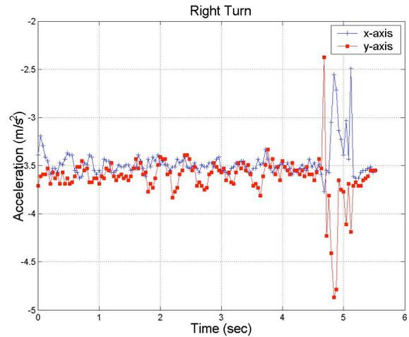
**Figure 3.** Acceleration data when the PipeProbe is making a right turn in an L-shape pipe fork. The right turn occurs around the 5th second.
