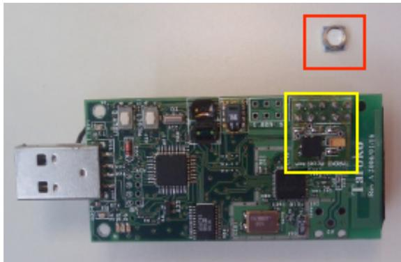
**Figure 1.** PipeProbe system with accelerometer module and pressure sensor module. The yellow rectangle marks the location of accelerometer module, and the red rectangle marks the pressure sensor module.
