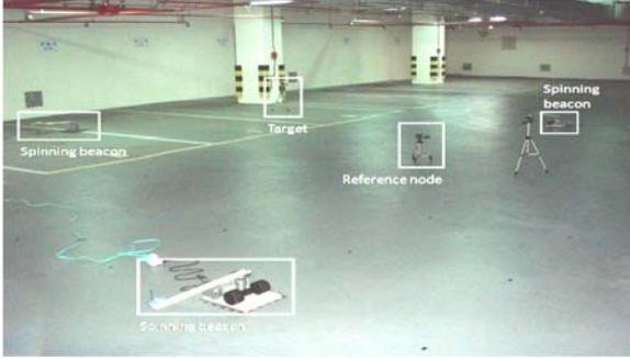
Figure 1. SpinLoc system deployment in a garage.
