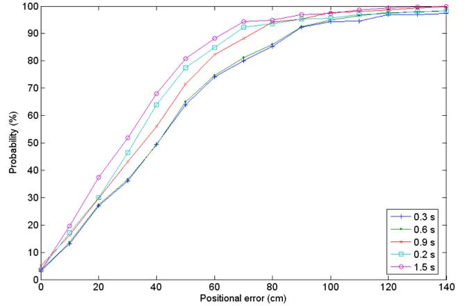
**Figure 18. CDF of the positional errors under different data collection times. The lines from right to left are in the order from 0.3s (top) to 1.5s (bottom) in the legends.**
