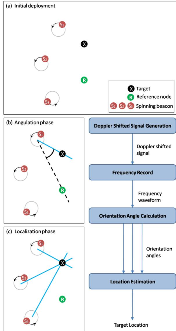
Figure 5. Deployment of the SpinLoc positioning system: (a) deployment layout, (b) angulation phase and (c) localization phase.
