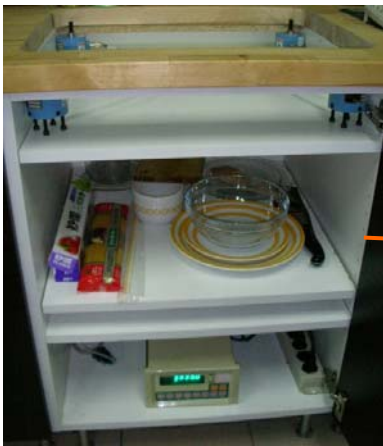
Weighing sensor deployment and space layout of smart counter (the upper line) and smart cabinet (the lower line)
