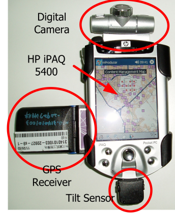
Figure 2: HP iPAQ 5400 with a digital camera, a GPS receiver and a tilt sensor
