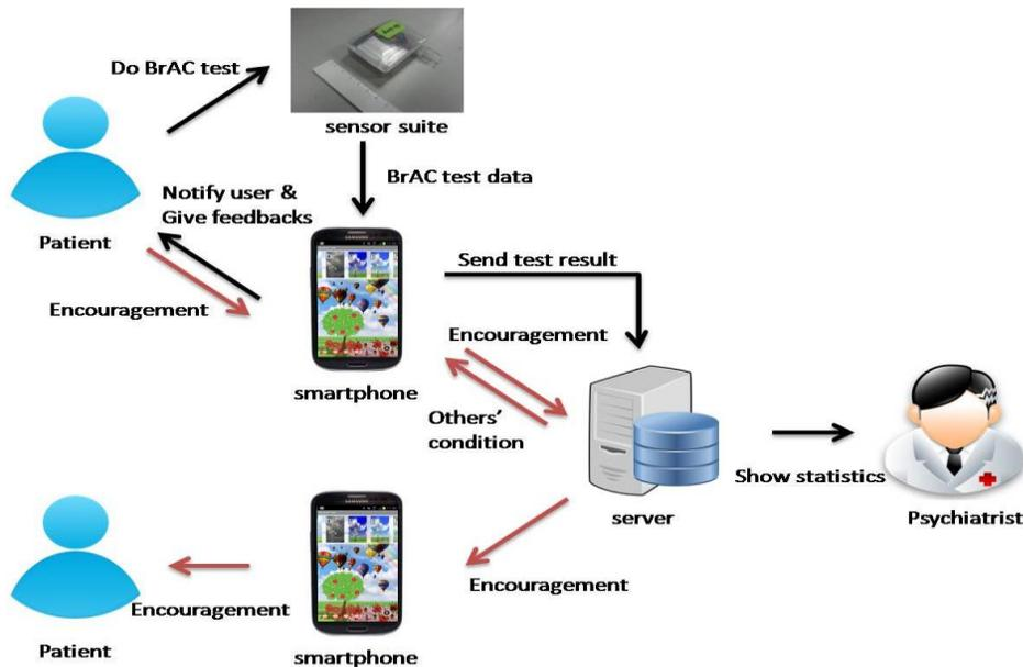
**Figure 1:** The system architecture. Black arrows represent the basic function of the system. Red arrows represent the interactive function of the system
