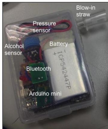
**Figure 2:** Sensor suite and main components. Note that the pressure sensor, Bluetooth and Arduino Mini are covered by battery.
