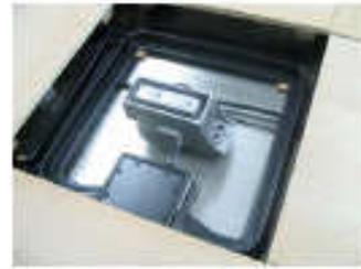
**Figure 2. The sensor surface on a smart kitchen counter. It is embedded with a weighing sensor and a RFID reader/antenna.**
