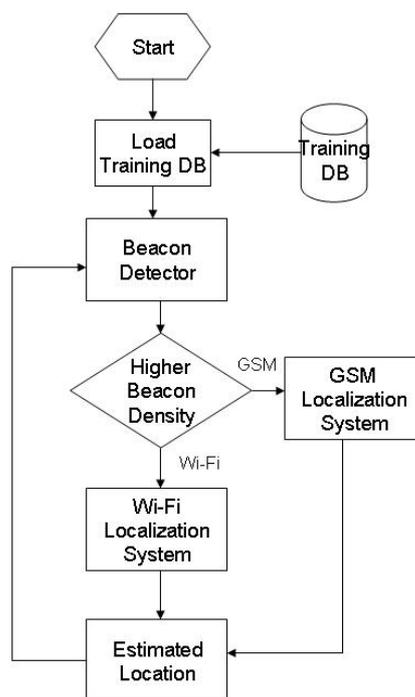
Fig. 33. System flow of GSM/Wi-Fi Hybrid Localization
