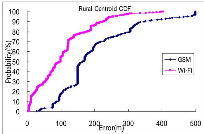
Fig. 16. CDF of GSM and Wi-Fi with Centroid Algorithm in rural area
