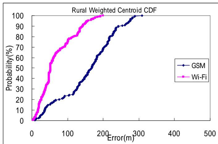
Fig. 17. CDF of GSM and Wi-Fi with Weighted Centroid Algorithm in rural area
