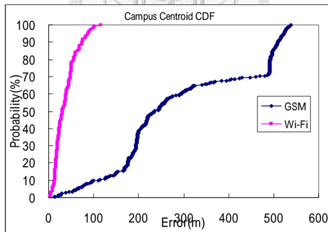
Fig. 22. CDF of GSM and Wi-Fi with Centroid Algorithm in campus
