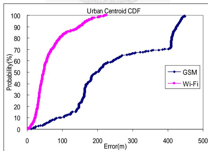
Fig. 10. CDF of GSM and Wi-Fi with Centroid Algorithm in urban area
