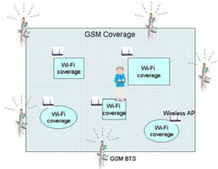
Fig. 32. A hybrid environment with different GSM or Wi-Fi density
