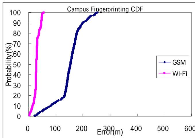
Fig. 24. CDF of GSM and Wi-Fi with Fingerprinting Algorithm in campus
