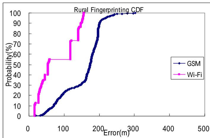
Fig. 18. CDF of GSM and Wi-Fi with Fingerprinting Algorithm in rural area
