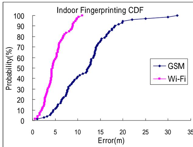
Fig. 28. CDF of GSM and Wi-Fi Indoor Fingerprinting in CSIE building
