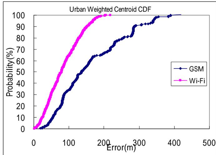
Fig. 11. CDF of GSM and Wi-Fi with Weighted Centroid Algorithm in urban area
