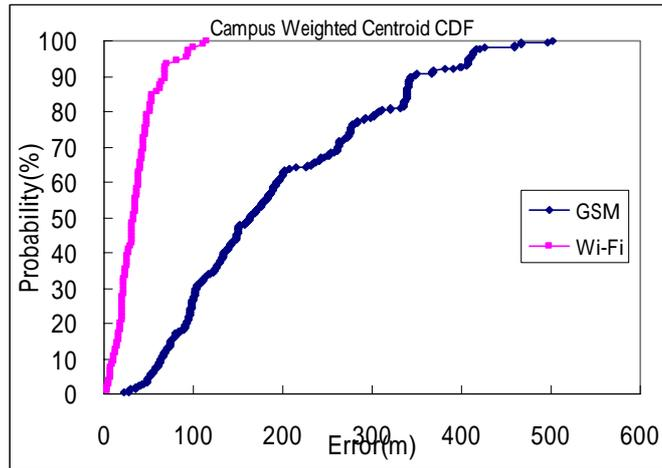
Fig. 23. CDF of GSM and Wi-Fi with Weighted Centroid Algorithm in campus
