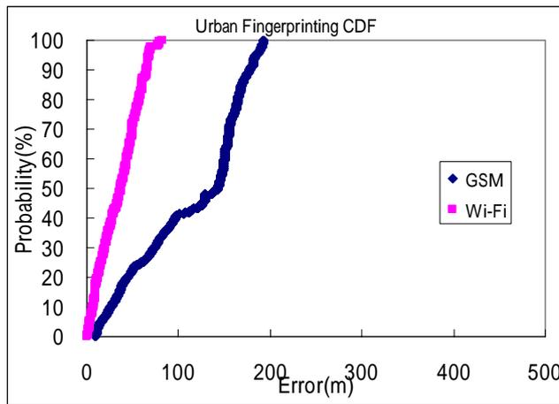
Fig. 12. CDF of GSM and Wi-Fi with Fingerprinting Algorithm in urban area
