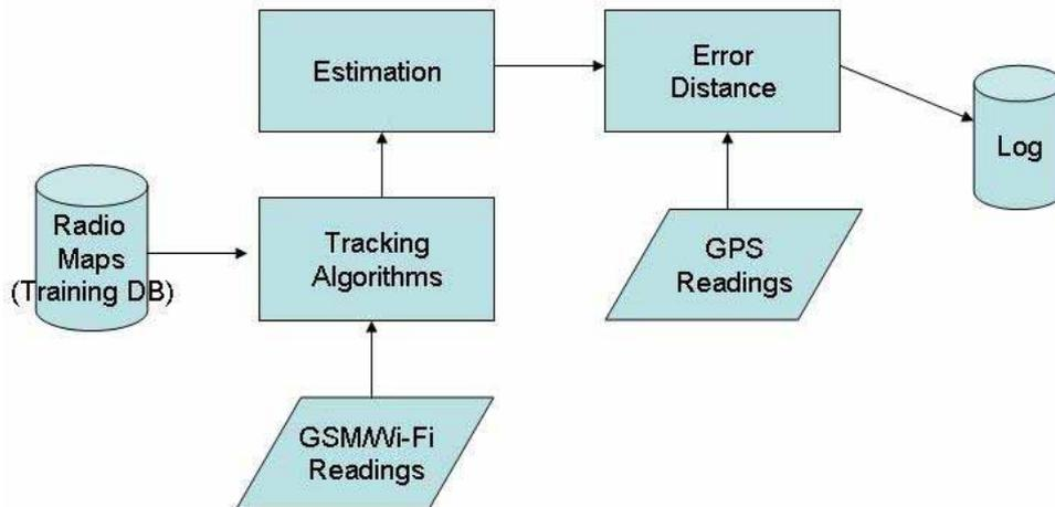
Fig. 6. System Architecture (Tracking)
