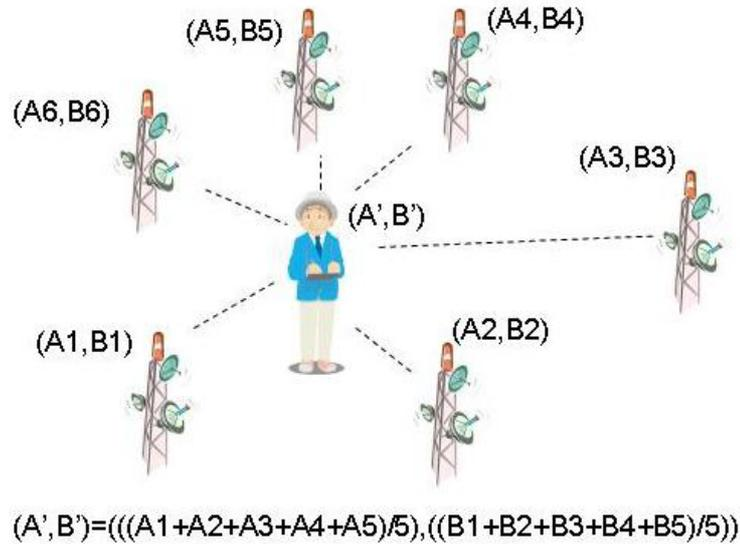
Fig. 2. Centroid Positioning (the coordinate of beacons is a prior knowledge)
