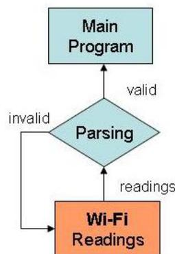
Fig. 8. Wi-Fi Implementation Diagram
