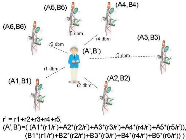
Fig. 3. Weighted Centroid Positioning
