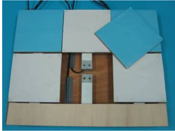
Figure 6.2: The smart lunch tray. The tray is divided into 2x3 cells, and each cell is embedded with a weight sensor. Only one food container can be put on a single cell.
