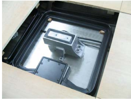
Figure 7.2: The sensors of a smart counter. The counter surface is embedded with a weighing sensor and a RFID reader/antenna.
