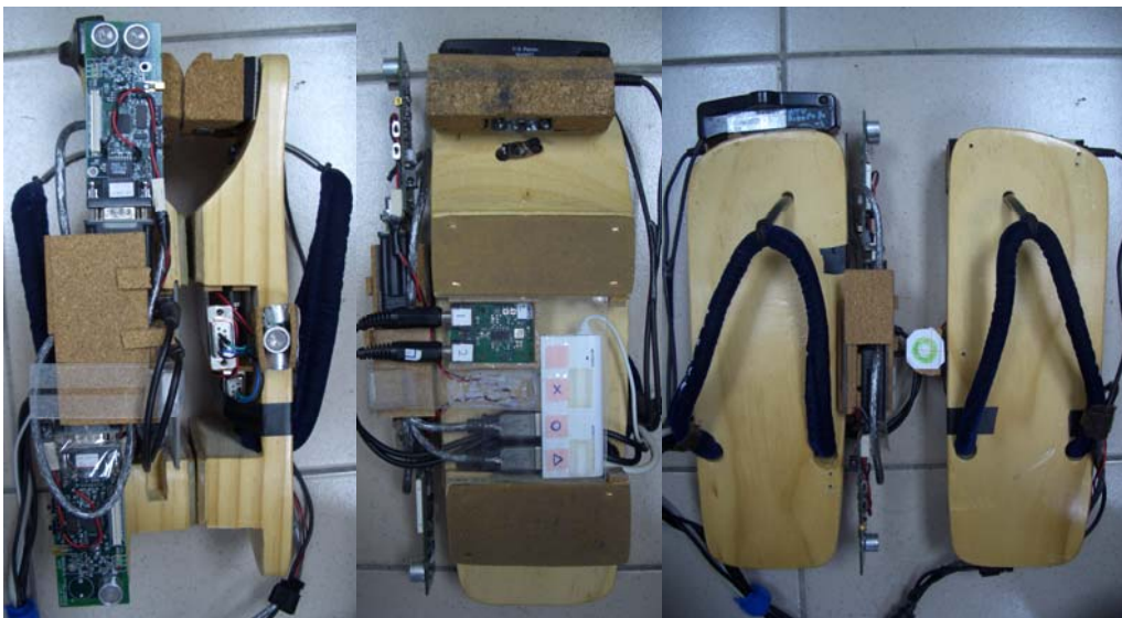
Fig. 9. The Second Prototype Implementation of GETA Sandals
